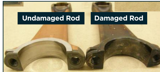
Recovered Pieces from Failed Rod Bearing
