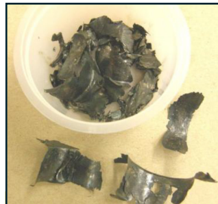
Recovered Pieces from Failed Rod Bearing
